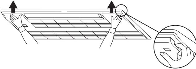
3. Pull the hinges and unhook the Safety strings to remove.
