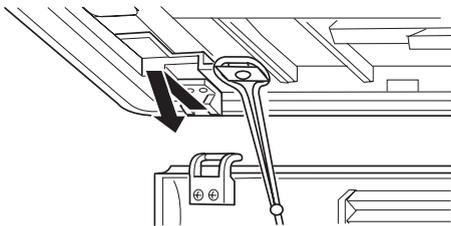
4. Install the intake grille by following the removal procedure in reverse. Close the intake grille securely and press the positions indicated by the arrows.
